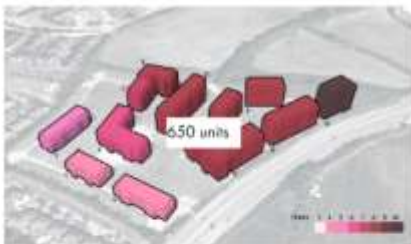
1. First scheme alteration- reduced heights (650 units). Number of levels have been reduced throughout all buildings. The extra units could be achieved by filling some gaps and extending some buildings.
